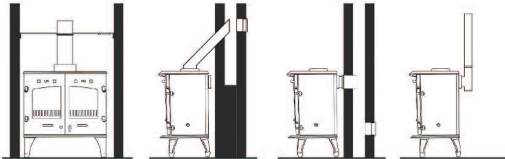
Attach the flue outlet to the stove with the screws and nuts provided. Use a steel closure plate to seal off the chimney; a cleaning door must be fitted into the plate or flue, and a steel sealing collar must be used to fit the flue into the steel plate. Seal all joints with fire cement.
